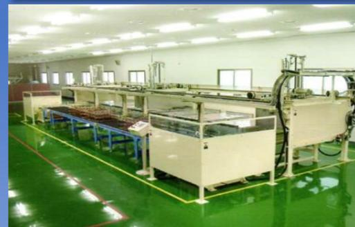
Cover glass for smartphones and other thin and small-sized glass that cannot be used with air-cooled reinforcement can be strengthened. No softening deformation or warpage due to reinforcement.
