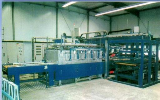
The air-cooled reinforcement unit enables reinforcement after bending, so it can be used for a wide range of applications such as building applications.
