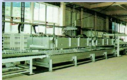
Air-cooled tempering equipment capable of producing tempered glass about three to five times that of ordinary flat glass. Can also be used for large sizes.
