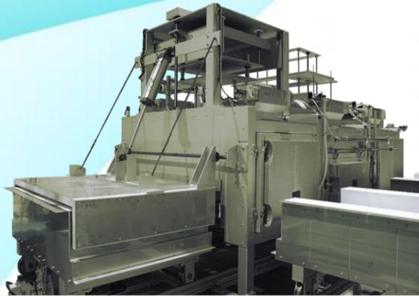
As the glass bending device for automotive instrument panel, it being applied by European automobile manufacturers.
